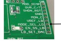
Alternatively, Mode control can be set by an external system. With the link in the CC/External position the control line can be accessed via Mod\_SEL\_LD at CN8. This node should be pulled high for Constant Power mode, and released, or pulled down, for Constant Current mode. (an internal pull-down inside the module sets Constant Current as the default mode).
