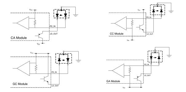
The MOT6550CA, CC and GA modules are characterized for dual supply operation, while the MOT6550GCmodules are characterized for single supply operation, with supply range from 3.3V to 5V.
