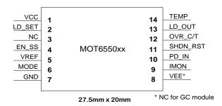
Laser current is continuously monitored and represented by a voltage at the monitor pin. This voltage can be measured using an external ADC and a microcontroller.
