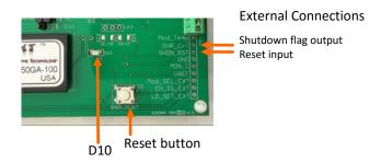
The shutdown functionality can also be monitored and restarted externally:
