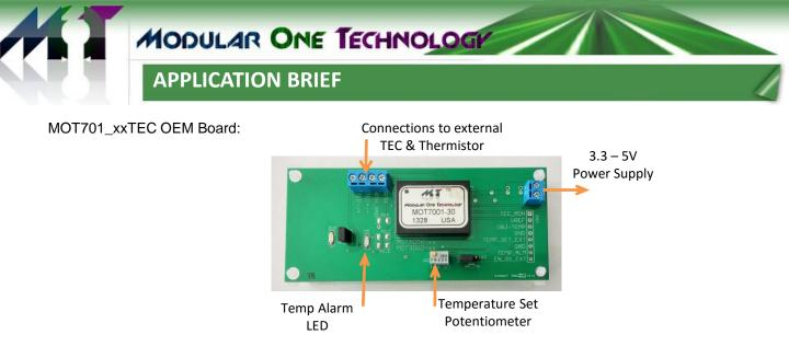
The above picture illustrates the minimal external connections needed with the application schematic built on the MOT701\_OEM board. This could be inserted into a suitable enclosure with power supply producing a complete Thermoelectric Cooler system!
