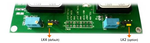
Alternatively the object temperature can be set by an external voltage applied to TEMP\_SET\_EXT on CN10. Pins 1 to 8 on CN10 connect to module 1 (U1) and pins 9 to 16 connect to module 2 (U2). The reference voltage, VREF, is also available on CN10 and can be used as a reference for an external DAC. In this mode LK2 & LK4 should be altered to the optional position.
