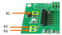
See the MOT700x data sheet for calculating values for R1, R2, and R3.
