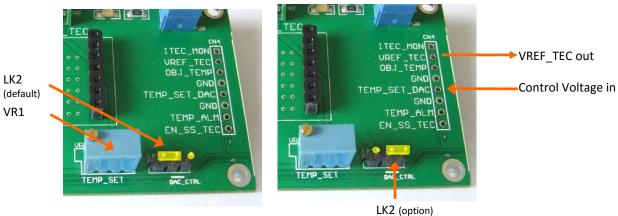
Alternatively the object temperature can be set by an external voltage applied to TEMP\_SET\_DAC on CN4. The reference voltage, VREF\_TEC, is also available on CN4 and can be used as a reference for an external DAC. In this mode LK2 should be altered to the optional position.
