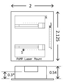
**Edge Connector** Laser Socket Pin Description Pin Number 1 TEC-9 8 2 Thermistor 3 Photodiode Anode 7 4 Photodiode Cathode 6 5 Thermistor 5 NC 6 7 Photodiode Cathode 6 8 Photodiode Anode 7 9 Laser Cathode 3 10 Laser Anode 4 Laser Cathode 3 11 12 NC 13 Case, GND 2 14 TEC+ 1
