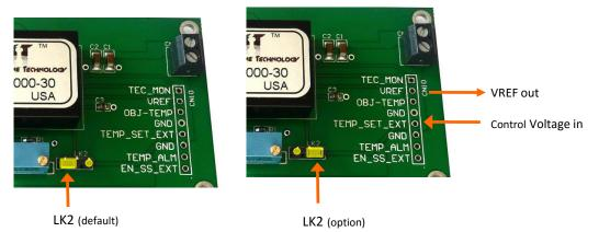
Alternatively the object temperature can be set by an external voltage applied to TEMP\_SET\_EXT on CN10. The reference voltage, VREF, is also available on CN10 and can be used as a reference for an external DAC. In this mode LK2 should be altered to the optional position.
