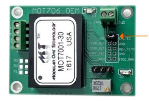
Module output enable/disable (pull high VCC to disable) Remove link to enable
