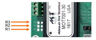
See the MOT700x data sheet for calculating values for R1, R2, and R3.
